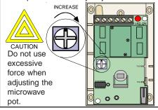
**3.11 Walk test the detector.** Perform this test at the time of installation and annually thereafter.
